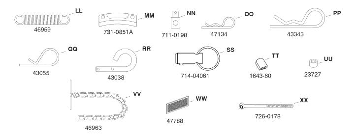
**IMPORTANT:** Not all items supplied in the hardware bag will be needed for your particular tractor. Unneeded items may be discarded after you have completed assembly and checked operation of unit. **DO NOT DISCARD** the two spare shear bolts (K) and 5/16" nylock nuts (HH). Refer to the Service and Adjustments section on page 18.
